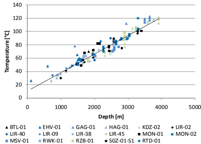
**Figure 2.** Measured BHT in seventeen wells. The solid line is the linear regression curve.
