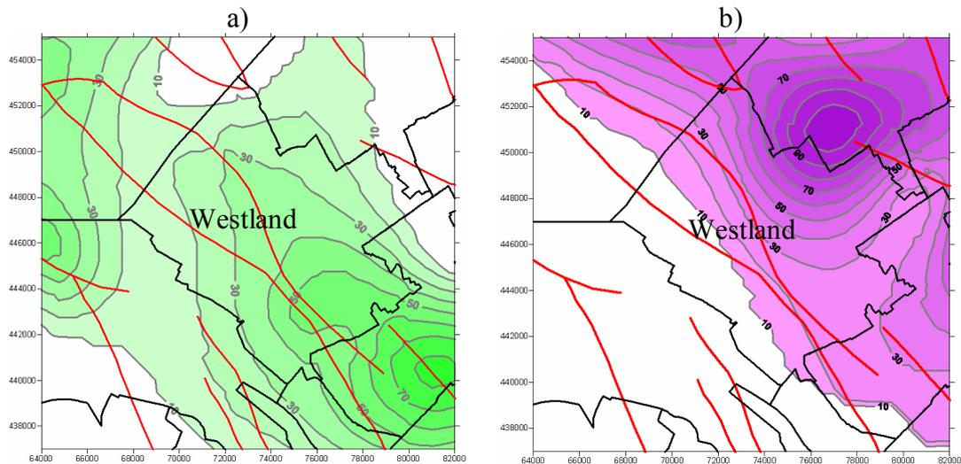
**Figure 3.** Reservoir thickness distribution at Westland. a) Berkel Sandstone Member, b) Delft Sandstone Member. Red lines denote the faults. Boundaries of Westland are delineated in black.
