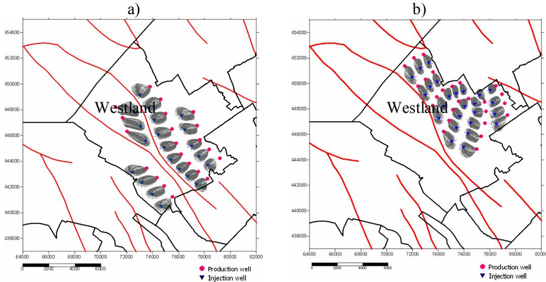
**Figure 4.** Well field design. a) Berkel Sandstone Member, b) Delft Sandstone Member. Red lines denote the faults. Boundaries of Westland are delineated in black.
